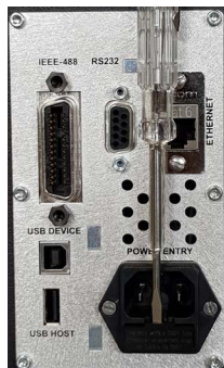
Fig. 10.1.2-A Position of the fuses
